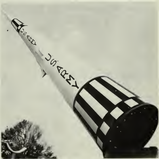
ANTI-MISSILE MISSILE Sprint , under advanced development by Army, will complement Zeus in Nike-X system.
